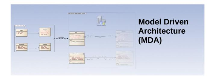
Enterprise Architect provides the capability of executing MDA transforms. It provides a fully configurable method of converting model elements and model fragments from one domain to another. This typically involves converting Platform-Independent Model (PIM) elements to Platform-Specific Model (PSM) elements. A single element from the PIM could be responsible for creating multiple PSM elements across multiple domains.
